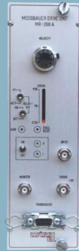
MR-260A Mössbauer Drive Unit with error minimisation facility and error display
