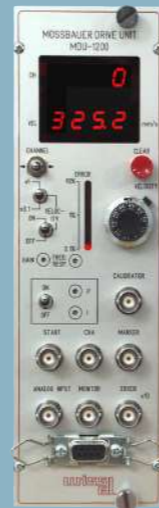
MDU-1200 Mössbauer Drive Unit with error minimisation, error display and velocity display based on laser calibration
